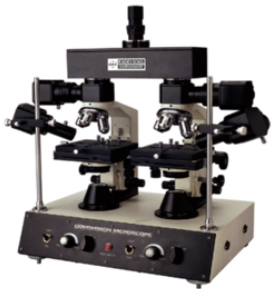
Fig. 5: Virtual comparison microscope which can be used to compare two specimens simultaneously 20
